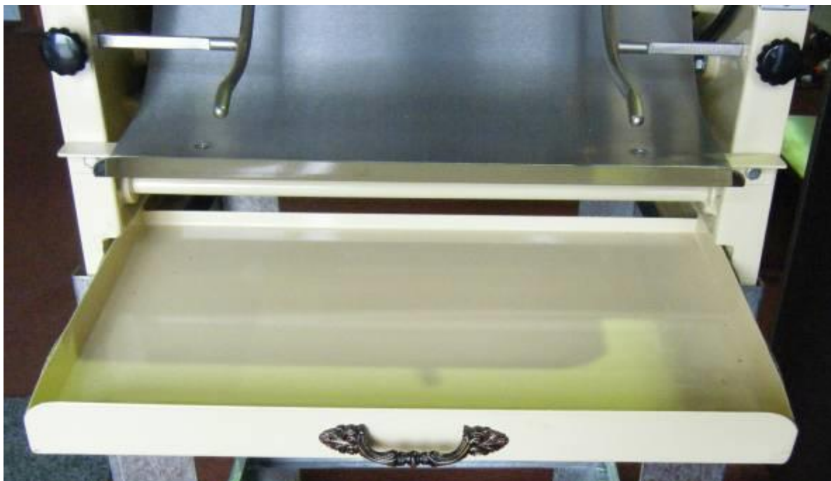
Fig1.3 Bread crumb draw, pulled out.
