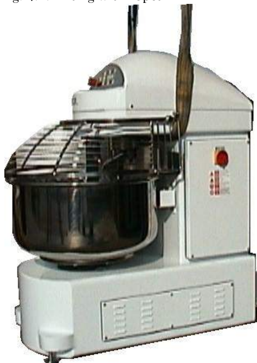
Fig. 4.1: Lifting with ropes
