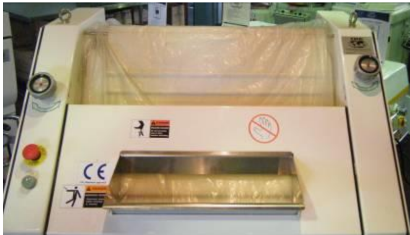
Fig1.3 In-feed chute in operating position
