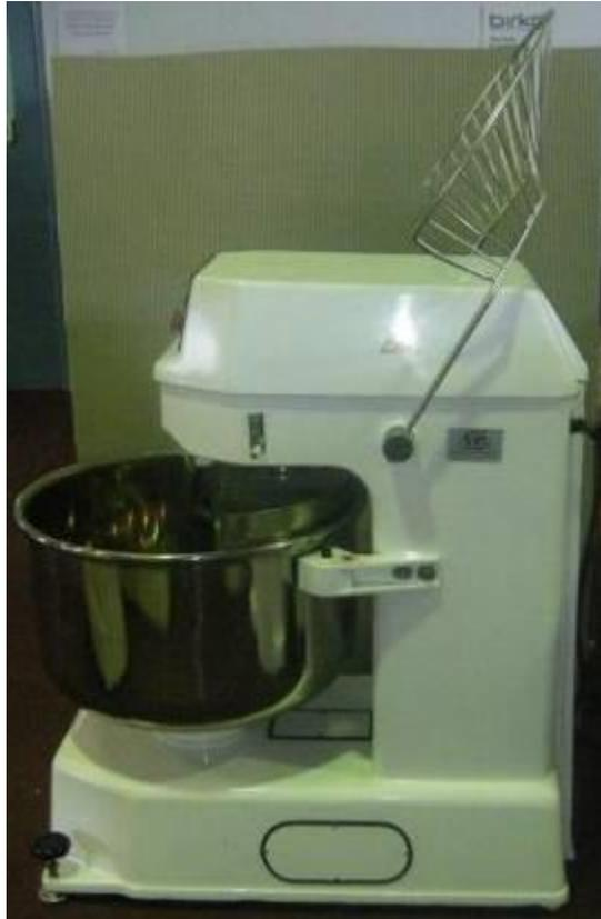
Fig1.7 Safety guard in raised position
