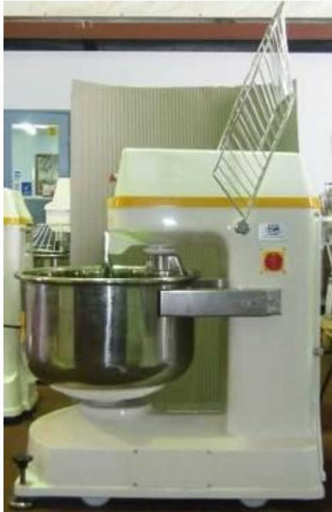
Fig1.7 Safety guard in raised position
