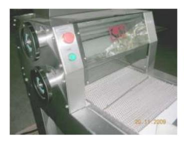
The most dangerous parts of the moulder machine are rollers.
