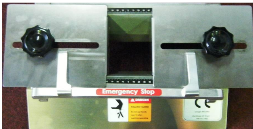
Fig1.3 In feed chute showing Emergency Stop Bar.
