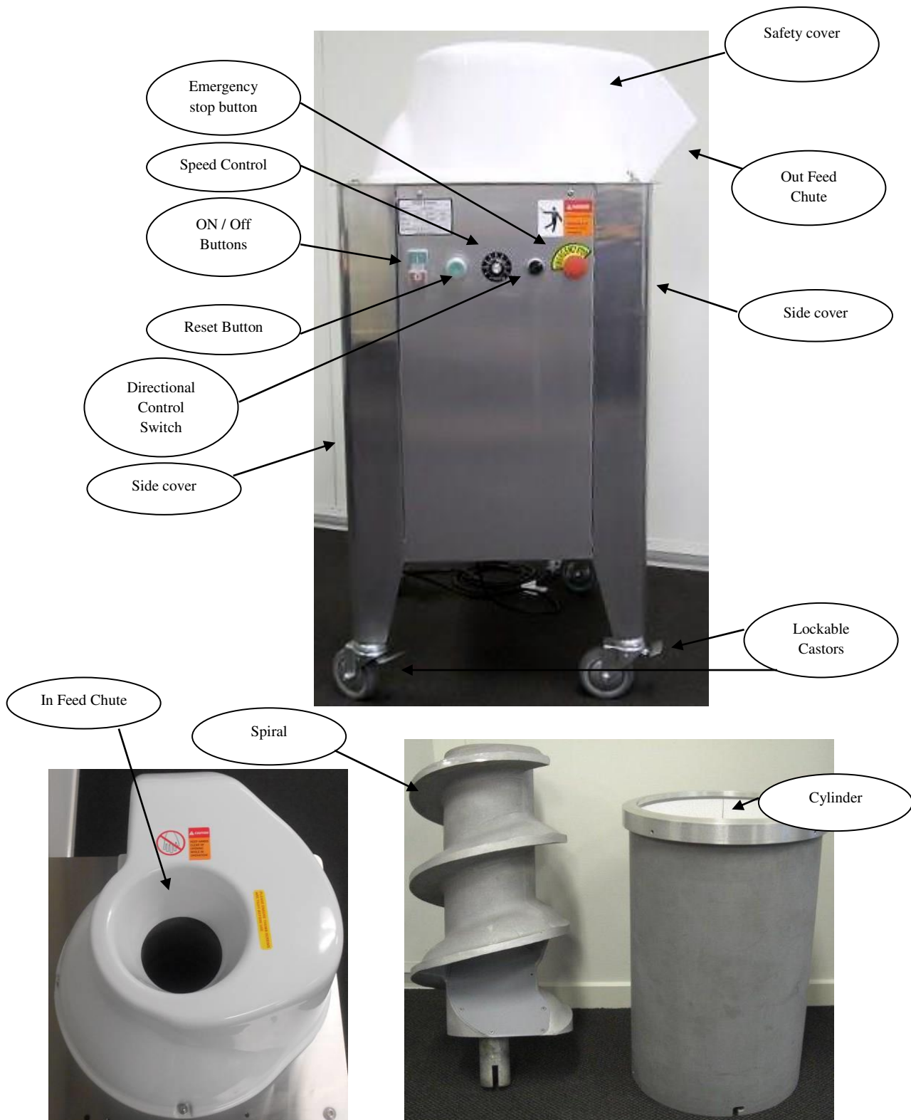
Fig1.2 Main Machine Components
