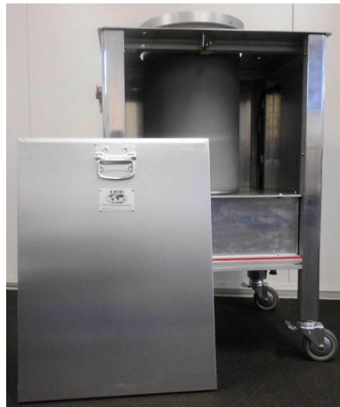
Fig1.3 The safety cover showing the locating pin, and side cover removed.
