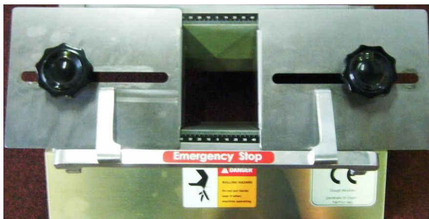
Fig1.3 In feed chute showing Emergency Stop Bar.
