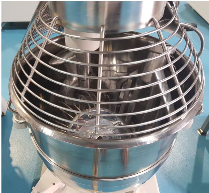
Fig 1.7 Safety guard in closed position
