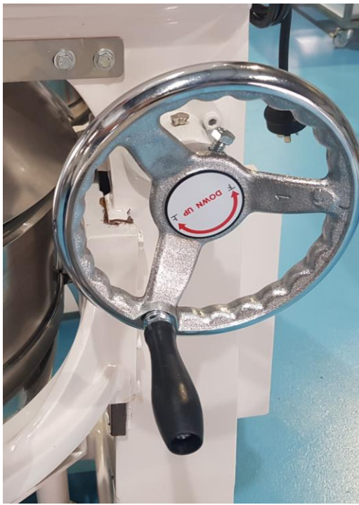
Fig 1.8 Bowl lift cradle in the raised position.
