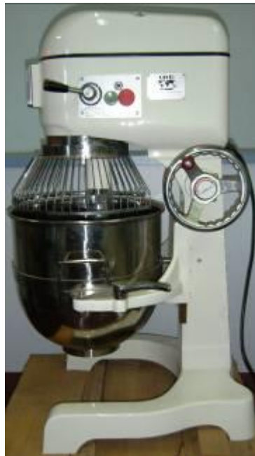
Fig 1.8 Bowl lift cradle in the raised position.
