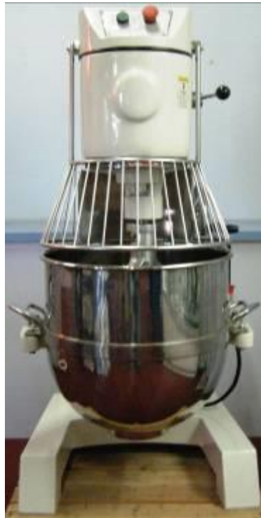
Fig1.7 Safety guard in closed position
