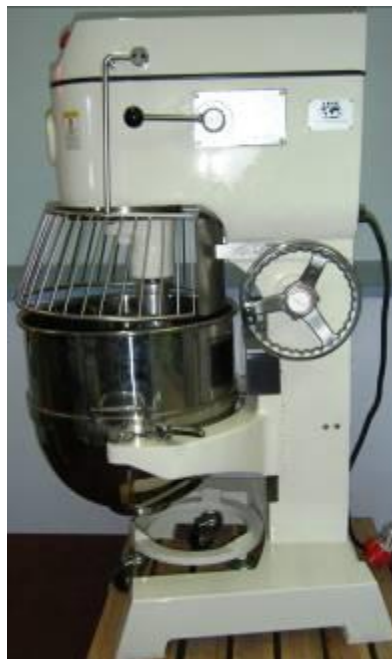
Fig 1.8 Bowl lift cradle in the raised position.
