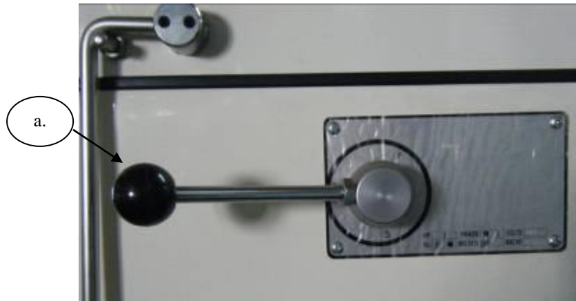
Fig 3.1 TM60B Gear selector
